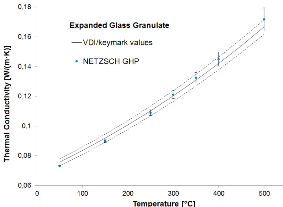
3 Thermal conductivity of an expanded glass granulate measured by means of the NETZSCH GHP 456 Titan® in comparison with the published VDI/keymark values (solid line). The dotted lines represent the standard uncertainty of the VDI/keymark values ( $\pm 3\%$ ) while the error bars reflect the combined standard measurement uncertainties.
