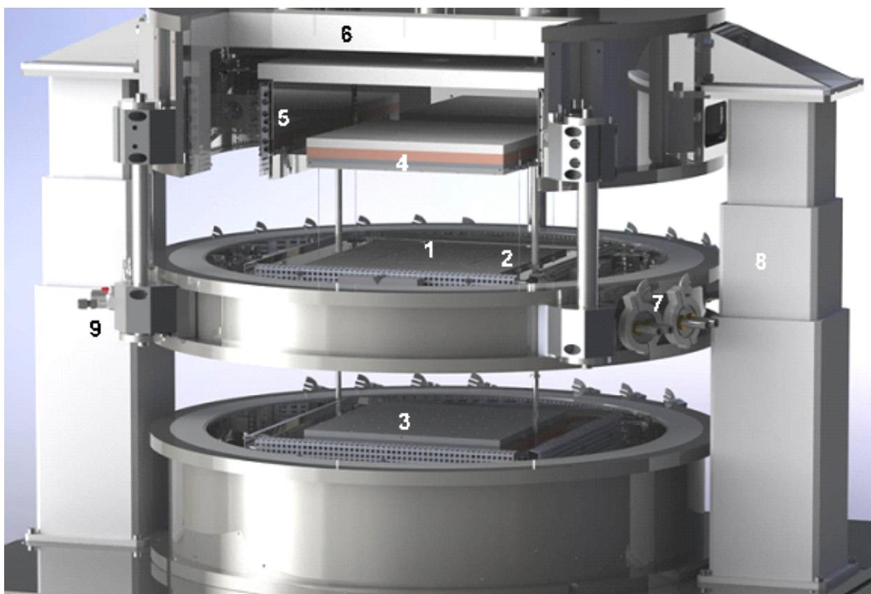
**1** NETZSCH GHP 456 *Titan*<sup>®</sup> in open position. A sample or two identical samples (not shown) are located between the hot plate (1) and guard ring (2) and the lower (3) and upper cold plates (4), respectively. Additionally shown are the three-part surrounding furnace (5), insulation (6), feed-throughs (7), hoisting device (8) and gas connection (9).
