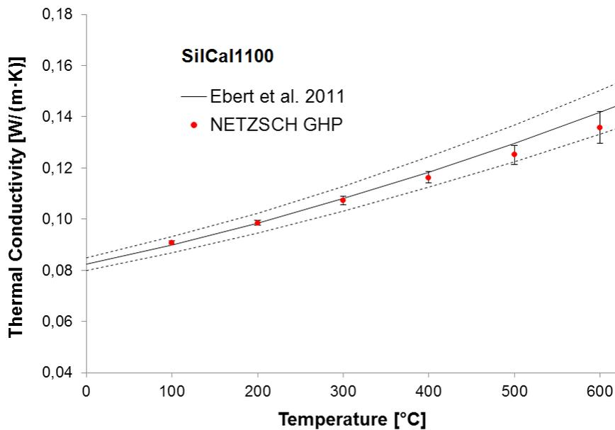
4 Thermal conductivity of SiCal1100, measured by means of the NETZSCH GHP 456 *Titan*® in comparison with the published round-robin values (solid line). The dotted line represent the standard uncertainties of the round-robin values ( $\pm 3\%$  increasing up to  $\pm 7\%$ ) while the error bars reflect the combined standard measurement uncertainties.
