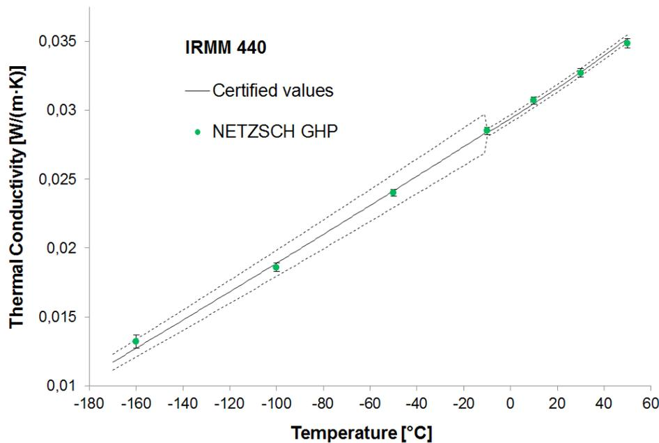
2 Thermal conductivity of IRMM 440, measured with the NETZSCH GHP 456 Titan® in comparison with the values certified by IRMM (solid line). The dotted lines represent the extended uncertainty budget of the IRMM values ( $\pm 5\%$  below  $-10^\circ\text{C}$ ,  $\pm 1\%$  above  $-10^\circ\text{C}$ ), while the error bars reflect the combined standard measurement uncertainties.
