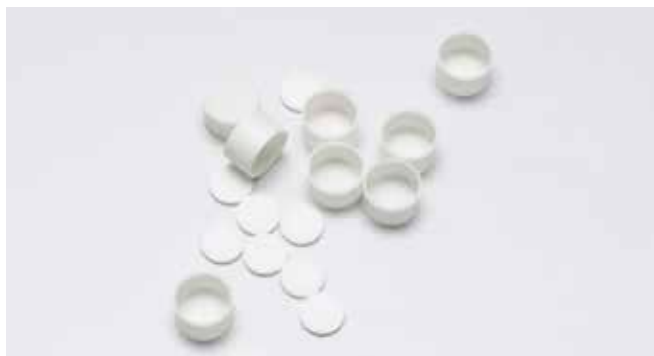
Fig. 3. \text{Al}_2\text{O}_3 crucibles and discs for measurement of powders with the TMA
