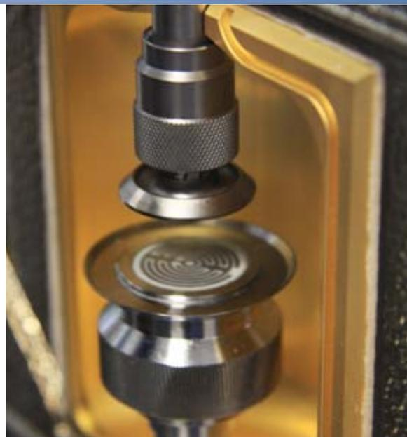
Fig.1: Parallel plates geometry with integrated DEA comb sensor in a temperature chamber for the HAAKE MARS rheometer.
