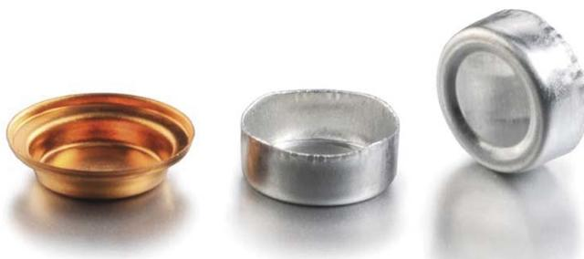
11 Copper (left) and aluminum crucibles (right), especially for determination of the OIT
