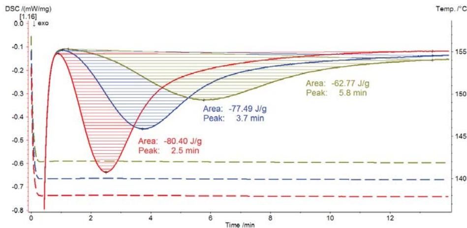
2 Isothermal crystallization of polypropylene at 3 different temperatures with the DSC 214 *Polyma* in a nitrogen atmosphere
