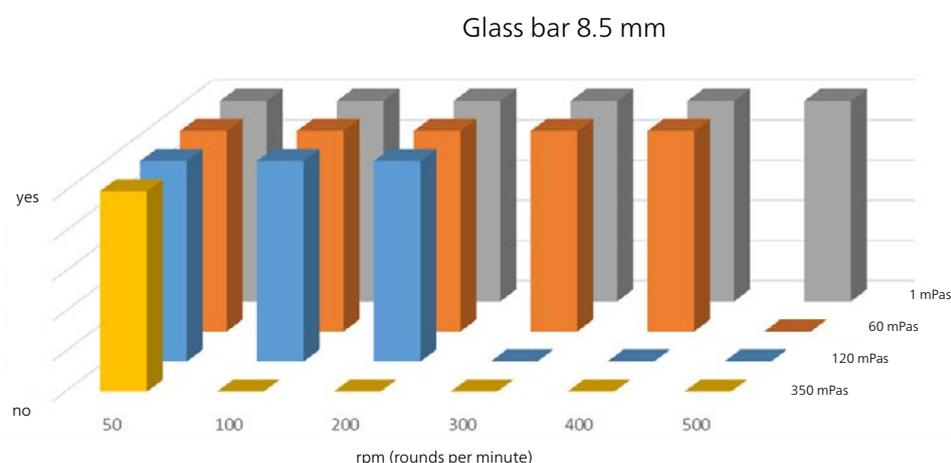
5 Efficiency of stirring inside the ARC® 254 using different media and varying rotation speed for a glass-coated stirring bar of 8.5 mm
