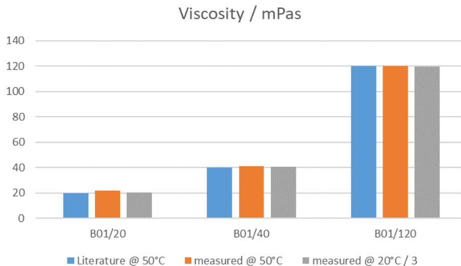
4 Comparison of the results for viscosity for three polyglycols measured with the NETZSCH Kinexus rotational rheometer. For better comparison, all values at 20°C (grey) are divided by 3.
