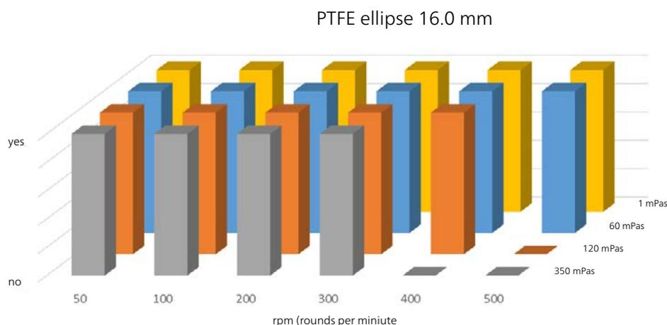
6 Efficiency of stirring inside the ARC® 254 using different media and varying rotation speed for a PTFE-coated, ellipsoid-shaped stirring bar of 16 mm
