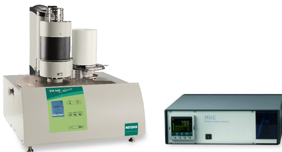
1 STA 449 F3 Nevio and modular humidity generator
