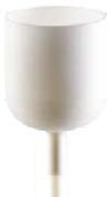
2 Alumina beaker crucible with a volume of 5 cm<sup>3</sup> for TGA measurements using NETZSCH STA 449 instruments
