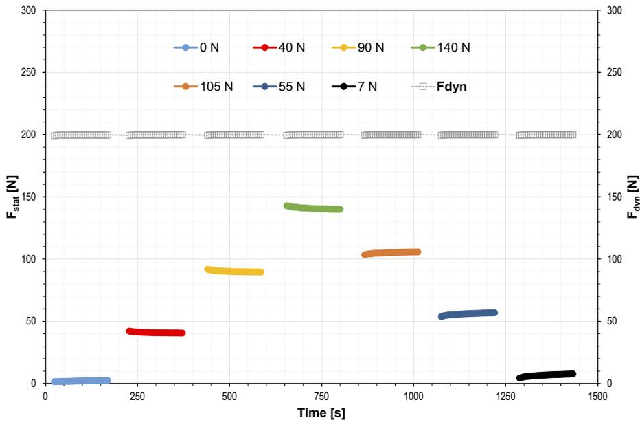
3 Temporal profile of the static and dynamic loads applied during the measurement
