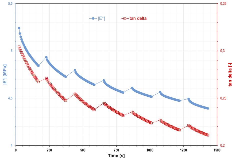
**5** Dependence of the modulus of elasticity (left) and loss factor (right) on time for the rubber-metal buffer with one stud bolt and one threaded hole at room temperature and a frequency of 10 Hz
