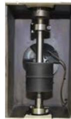
2 Mounted rubber-metal buffer with one stud hole and one threaded hole on the High-Force DMA GABO EPLEXOR®
