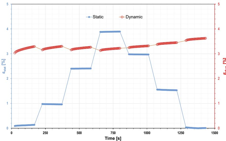
4 Variation of the static and dynamic strain over time for the rubber-metal buffer with one stud bolt and one threaded hole
