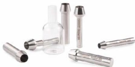
2 Sample vessels for the NETZSCH MMC 274 *Nexus*®
