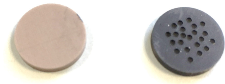
3 Filled polymer disc on the left, polymer disc with boreholes on the right
