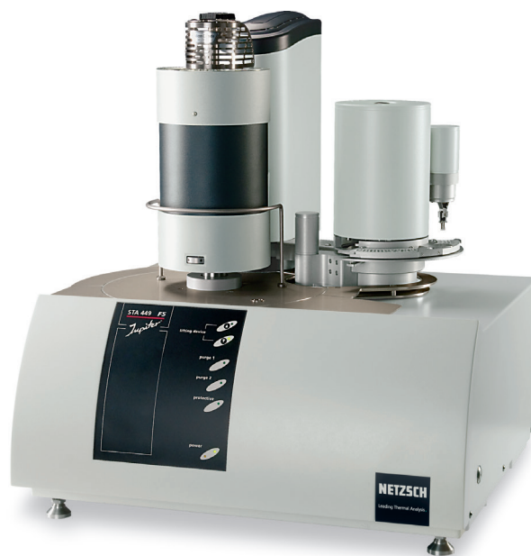
1 NETZSCH STA 449 F5 Jupiter ® equipped with an optional automatic sample changer (ASC)
