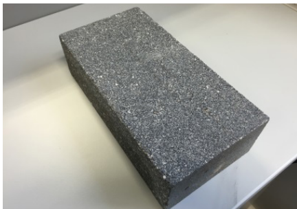
6 Silicone carbide-containing brick (45% Al 2 O 3 , 29% SiO 2 , and 25% SiC), measured with the TCT 426 (left) and LFA 427 (right); the 3 LFA samples were coated with graphite.
