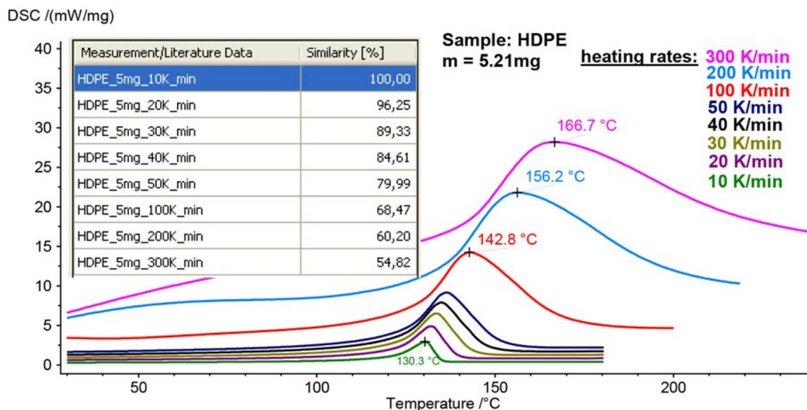
3 DSC curves (2<sup>nd</sup> heatings) of a HDPE sample measured at different heating rates of 10, 20, 30, 40, 50, 100, 200 and 300 K/min using a NETZSCH DSC 214 *Polyma*. The table shows similarity values from *Identify* in relation to the curve obtained at 10 K/min.
