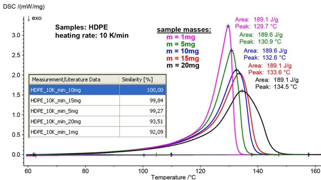
2 DSC curves (2<sup>nd</sup> heatings) of HDPE samples measured with different samples masses (1, 5, 10, 15 and 20 mg) using a NETZSCH DSC 214 *Polyma*. The table shows similarity values between the measurement for the 10-mg sample and the curves for the 1-, 5-, 15-, and 20-mg HDPE samples.
