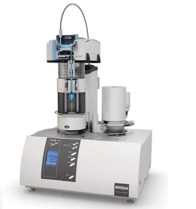
1 NETZSCH Perseus STA 449: The Bruker type "alpha" FT-IR spectrometer coupled directly to an STA 449 Jupiter simultaneous thermal analyzer equipped with an optional automatic sample changer (ASC). The sample space of the furnace, the heated coupling interface as well as the gas cell of the FT-IR spectrometer are shown partially transparent in order to display the path of the evolved gases [1].
