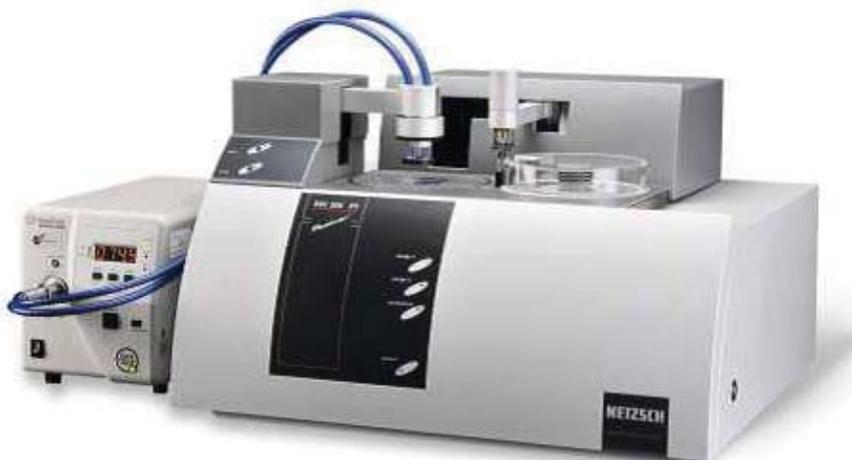
NETZSCH DSC 204 **F1 Phoenix**<sup>®</sup> with sample changer and OmniCure<sup>®</sup> 2000 mercury vapor lamp (other commercial UV lamps can also be used)
