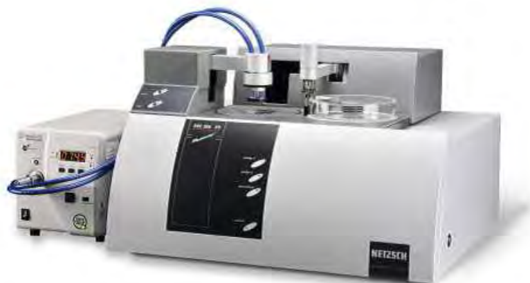
1 NETZSCH DSC 204 F1 Phoenix ® with OmniCure ® S2000 and light guide
