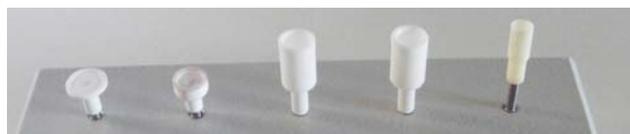
1 Al<sub>2</sub>O<sub>3</sub> crucible assortment (from left to right); slip-on plate, short DTA crucible, standard crucible, pierced DTA crucible, mini DTA crucible
