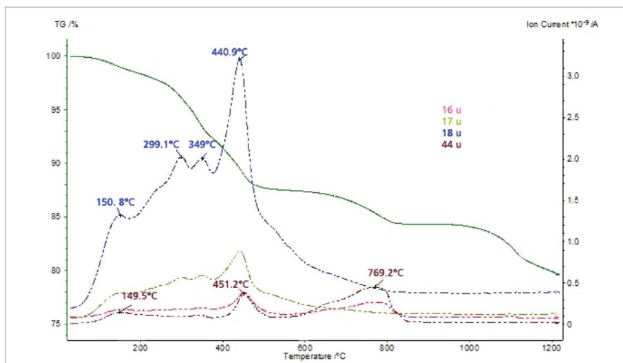
**4** MS ion-current curves for mass numbers 16, 17, 18 and 44 u and TGA curve for the thiol-capped ZnO nanoparticles sample
