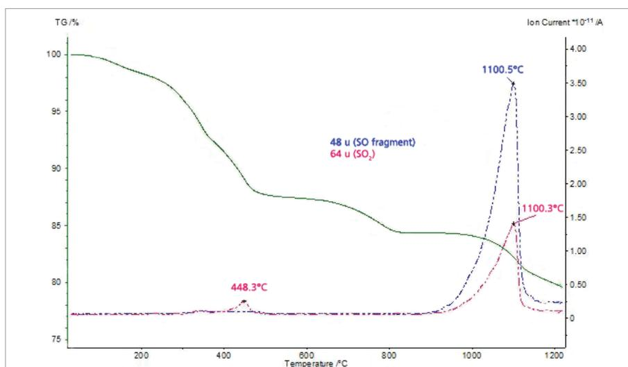
5 MS ion-current curves for mass numbers 48 and 64 u and TGA curve for the thiol-capped ZnO nanoparticles sample
