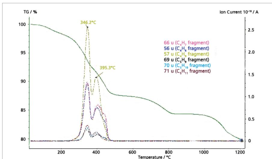
6 MS ion-current curves for mass number 55; 56; 57; 69; 70 and 71 u and TGA curve for the thiol-capped ZnO nanoparticles sample
