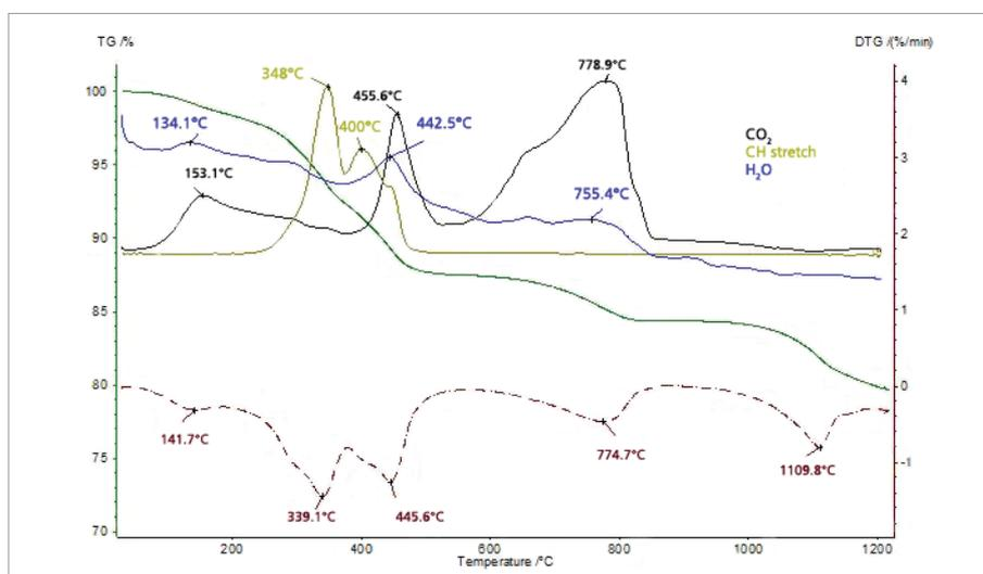
**3** TGA and DTG curves and the FT-IR traces for CO<sub>2</sub>, CH stretch and H<sub>2</sub>O for the thiol-capped ZnO nanoparticles sample
