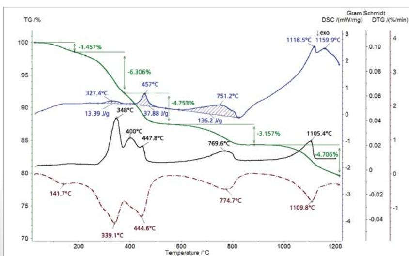
2 TGA, DTG, DSC and Gram Schmidt curves for the thiol-capped ZnO nanoparticle sample
