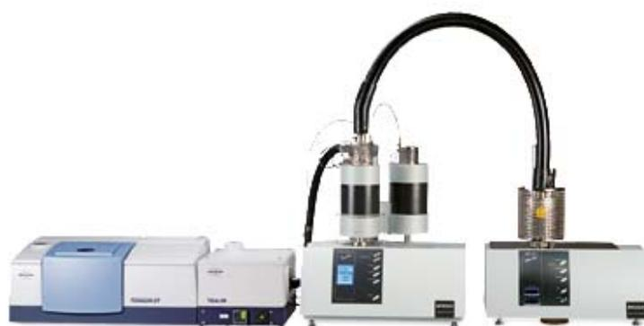
1 NETZSCH STA 449 **F1 Jupiter**<sup>®</sup> coupled to a NETZSCH QMS 403 **Aeolos**<sup>®</sup> and a BRUKER Optics TENSOR<sup>™</sup> FT-IR spectrometer
