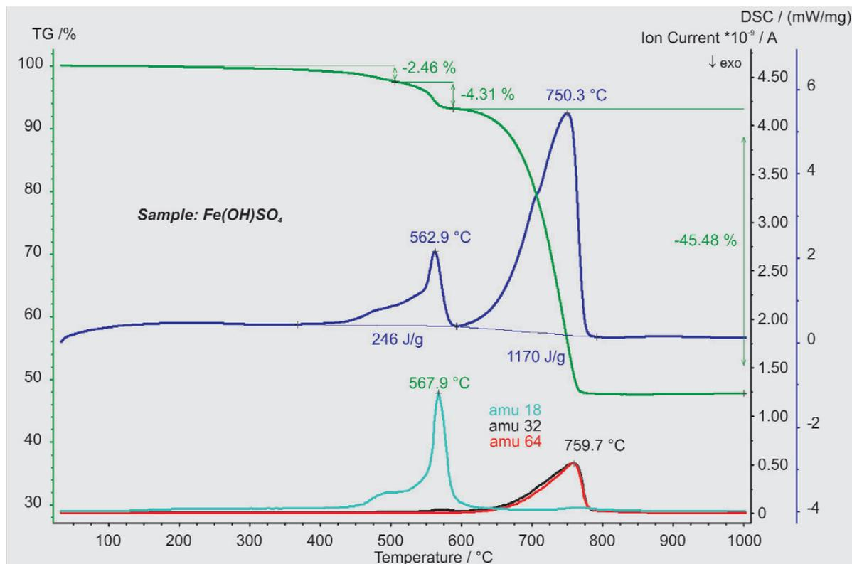
Fig 2. Mass change (TG), heat flow rate (DSC) and mass spectrometer curves (mass numbers 18, 32 and 64) of an  $\text{Fe(OH)SO}_4$  sample
