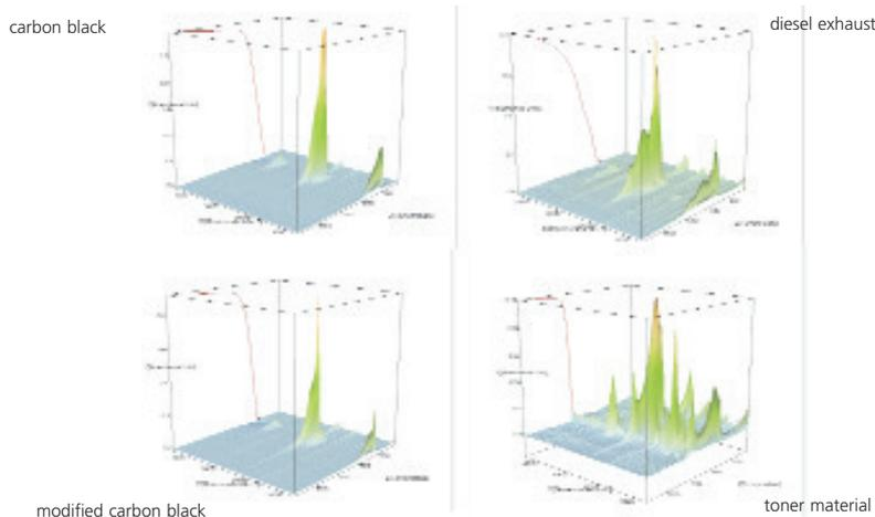
Fig. 3: Results of the TG measurements with subsequent FTIR analysis
