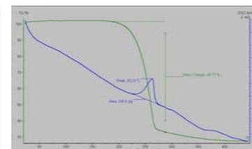
Figure 5. DSC and TG Curves of Sample 39
