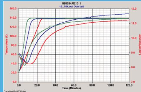
Fig. 6 : Comparison of the DEA measuring results for a PUR paint at different heating rates: 15 K/min (green), 10 K/min (blue) and 5 K/min (red)
