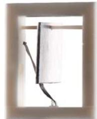
Sample holder for hanging samples, see also *Accessories for Differential Scanning Calorimeters and Thermobalances*
