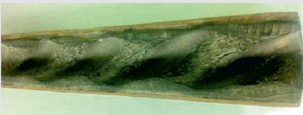
Fig. 01 - Stator damaged due to dry running
