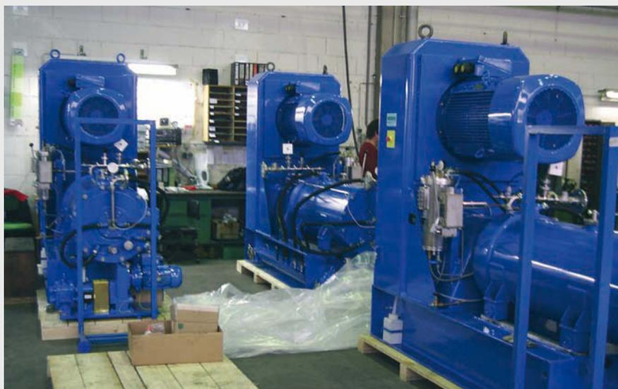
The LME Horizontal Bead Mills, with patented Dynamic Classifier System (DCC), provide increased throughput rates with virtually no blockage.
