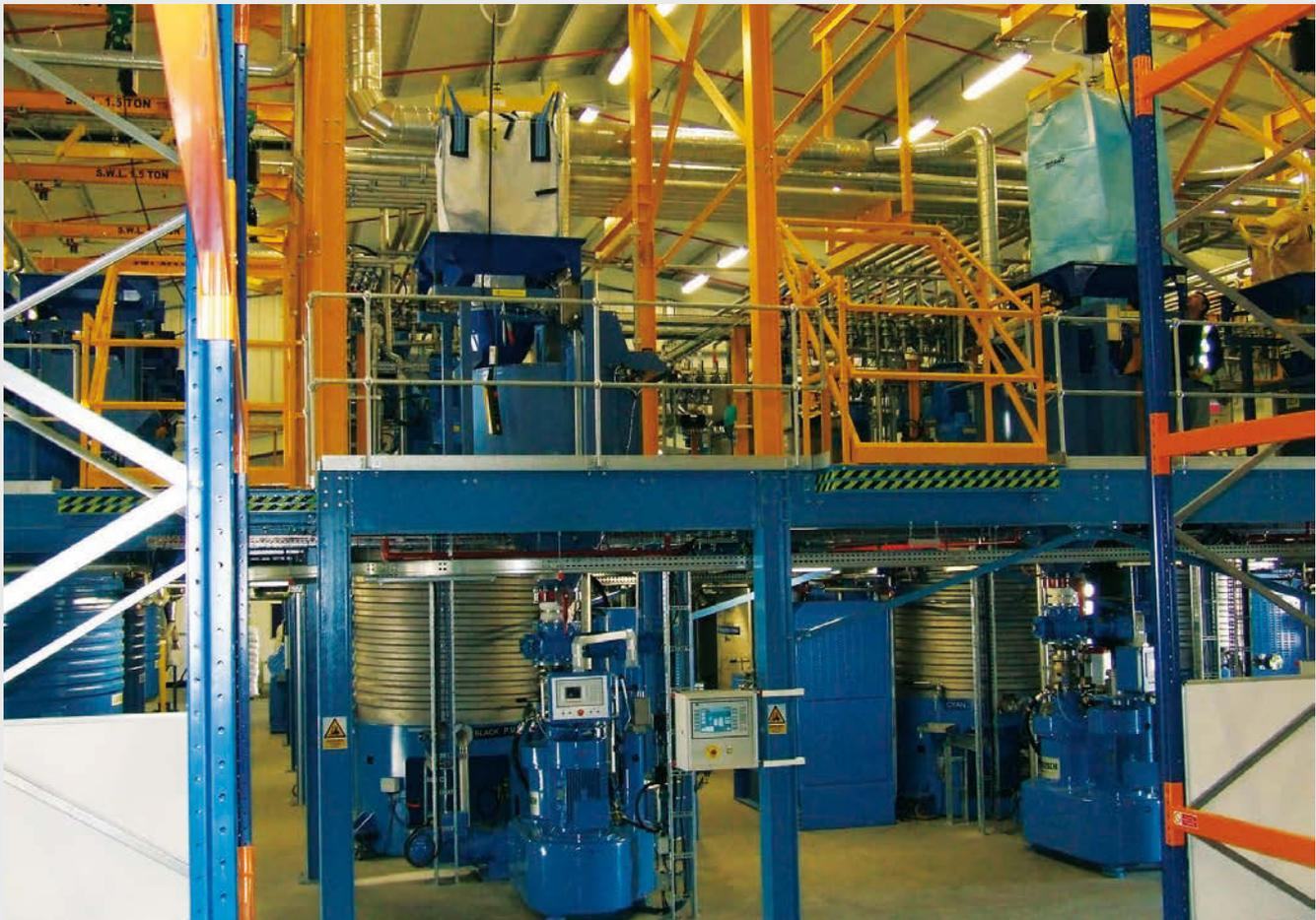
The revolutionary  $\Psi$ -Mix<sup>®</sup> used in the plant, with a combination of vacuum dispersing, shearing and pressure wetting resulted in high productivity, with excellent results and total reproducible quality.
