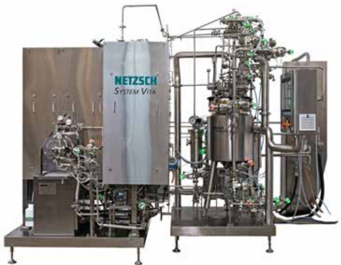
System VITA®, comprising a DELTAVITA ® agitator bead mill and a GAMMAVITA ® premix vessel
